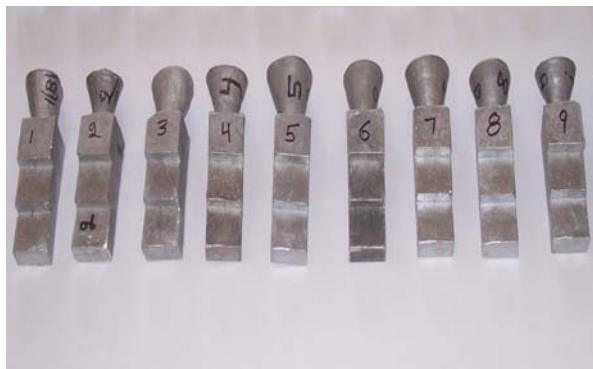
Fig. 3 Castings of Al-7%Si alloy
